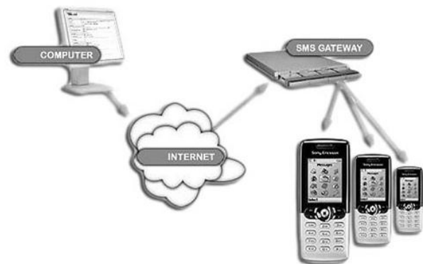
Figure.1: SMS Gateway system
