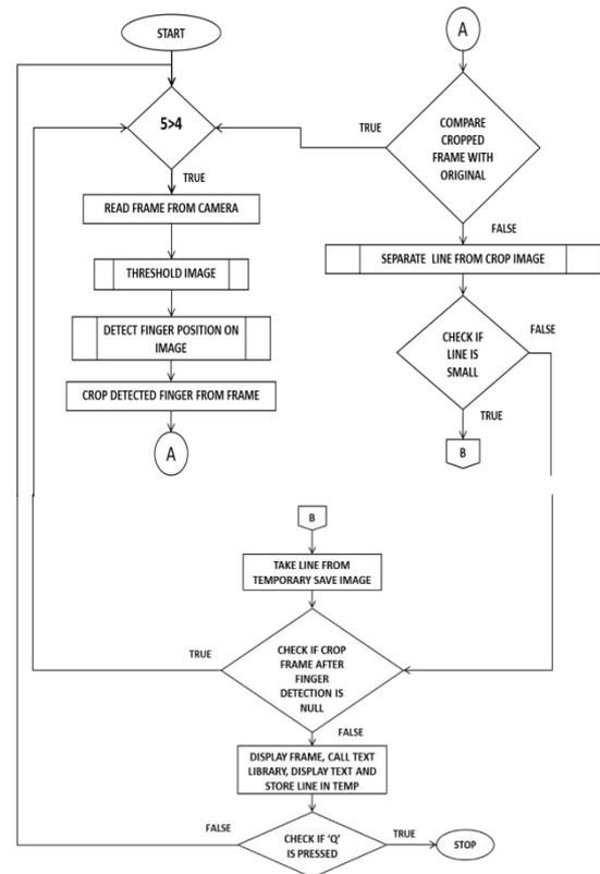
Figure.2: Flow diagram of the system.
