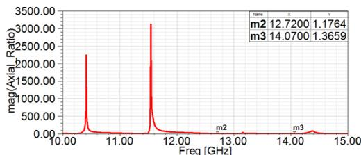
Figure 10: The axial ratio of transmitted wave versus frequency of dual-layer circular
