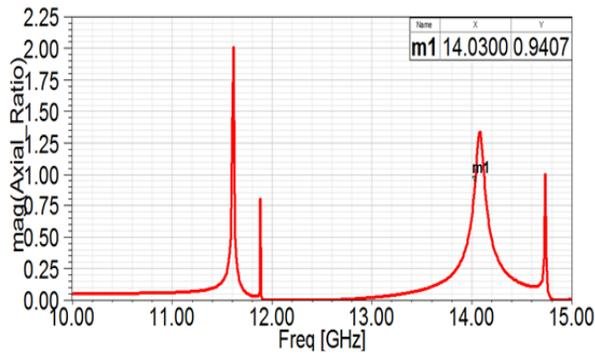
Figure 7: Simulated axial ratio versus frequency of single-layer.
