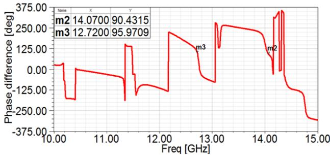
Figure 12: Phase difference of E-field versus frequency of dual-layer circular polarizer.
