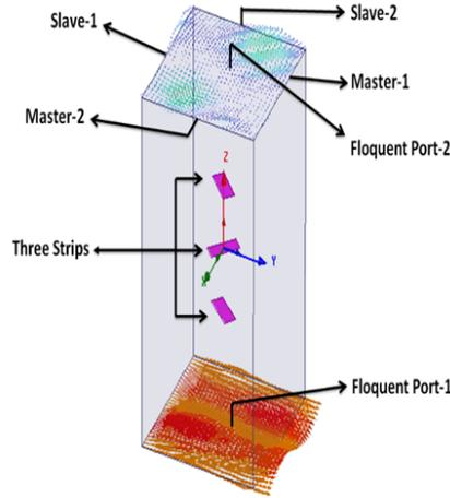
Figure6: Simulation model of three-layer circular polarizer
