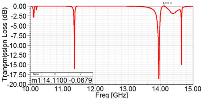
Figure 14: Transmission loss of E-field versus frequency of three-layer circular polarizer. The phase shift between transmitted wave  $E_x$  and  $E_y$  is to be 900.3 at the 14.11 GHz to realize linear-to-circular polarization as depicted in Figure 15.
