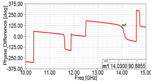
Figure 9: Phase difference of E-field versus frequency of single-layer circular polarizer
