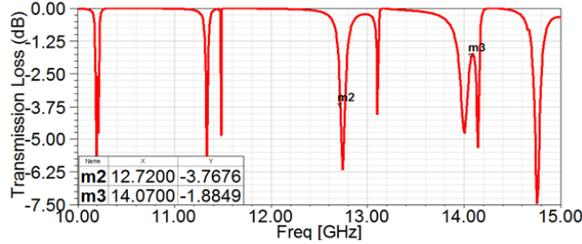
Figure 11: Transmission loss of E-field versus frequency of dual-layer circular polarizer. The phase difference of is noticed at 12.7 and at 14.07 GHz corresponding to fractional axial ratio of double-layer polarizer as denoted in Figure.12.
