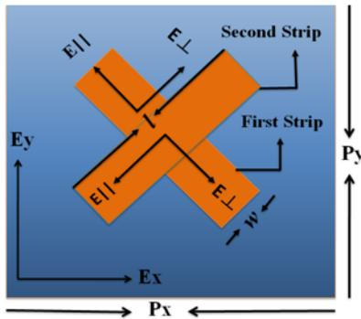
Figure 2: The schematic view of double-layer circular polarizer
