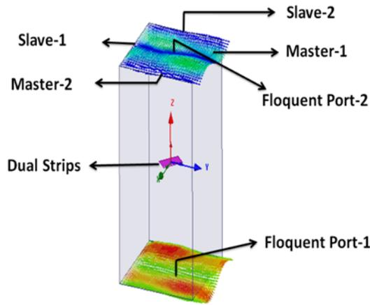
Figure4: Simulation model of single-layer circular polarizer
