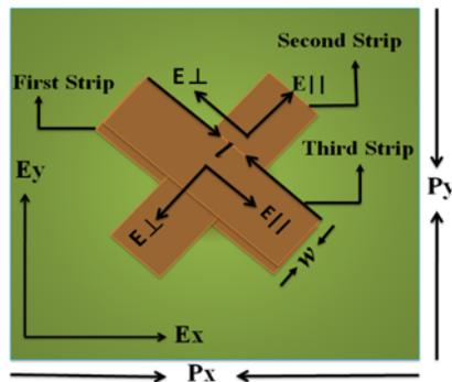
Figure 3: The schematic view of three-layer circular polarizer
