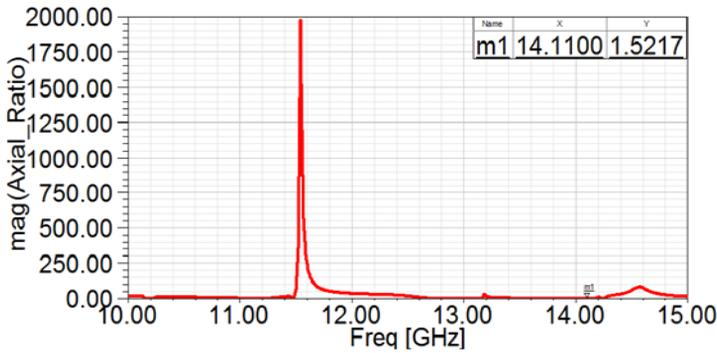
Figure 13: The axial ratio versus frequency of three-layer circular polarizer. It is noticed that the transmission loss and pass band of three layer polarizer has been improved than single and dual layer polarizer by adding three layer of strip. The structure demonstrates the transmission loss of -0.06 dB at the 14.11 GHz which is better than reported work as represented in Figure 14.
