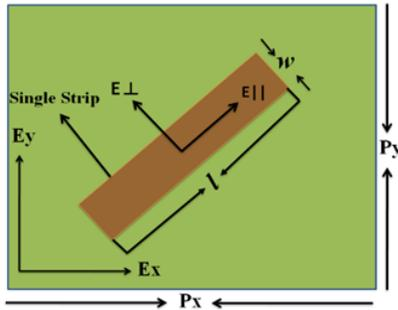
Figure 1: The schematic of single-layer circular polarizer
